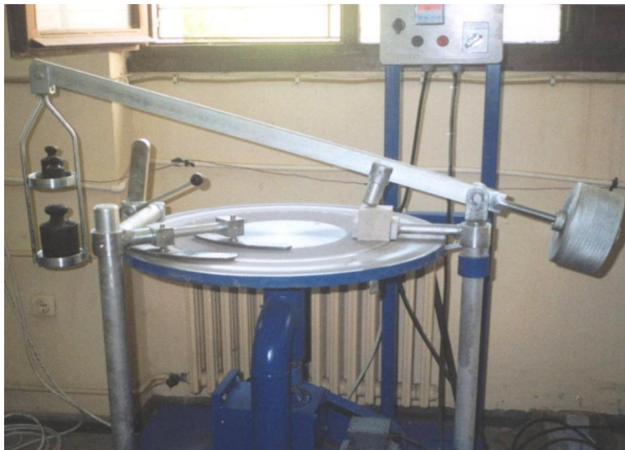
Figure 13. Photograph of Bohme abrasion test.
