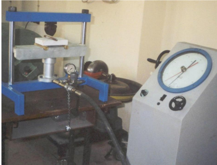
Figure 12. Photograph of strength to bending test.
